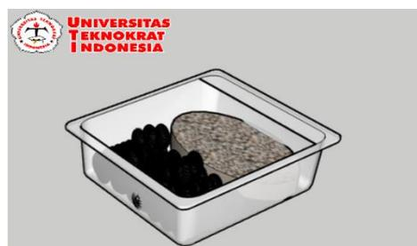
**Gambar 2.1** Biofilter Media Bio rings dan Bioball
