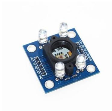
**Gambar 2.2** Sensor Warna TCS3200
