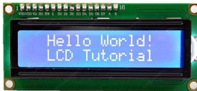
**Gambar 0.5** *Liquid Crystal Display*
