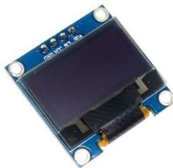
**Gambar 2.4** LCD OLED
