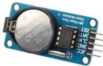
**Gambar 2. 3** Sensor RTC (*Real Time Clock*)
