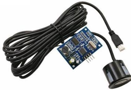
**Gambar 2. 6** Sensor Ultrasonic
