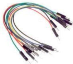
**Gambar 2. 7** Kabel Jumper
