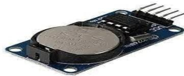
**Gambar 2. 7** Sensor RTC
