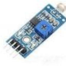
**Gambar 2.5** Modul LDR (*Light Dependent Resistor*)
