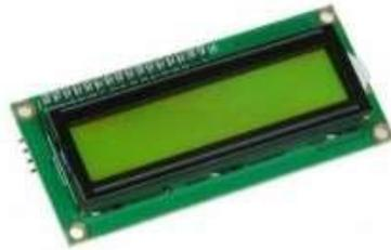
**Gambar 2.10** *Liquid Crystal Display* (LCD)
