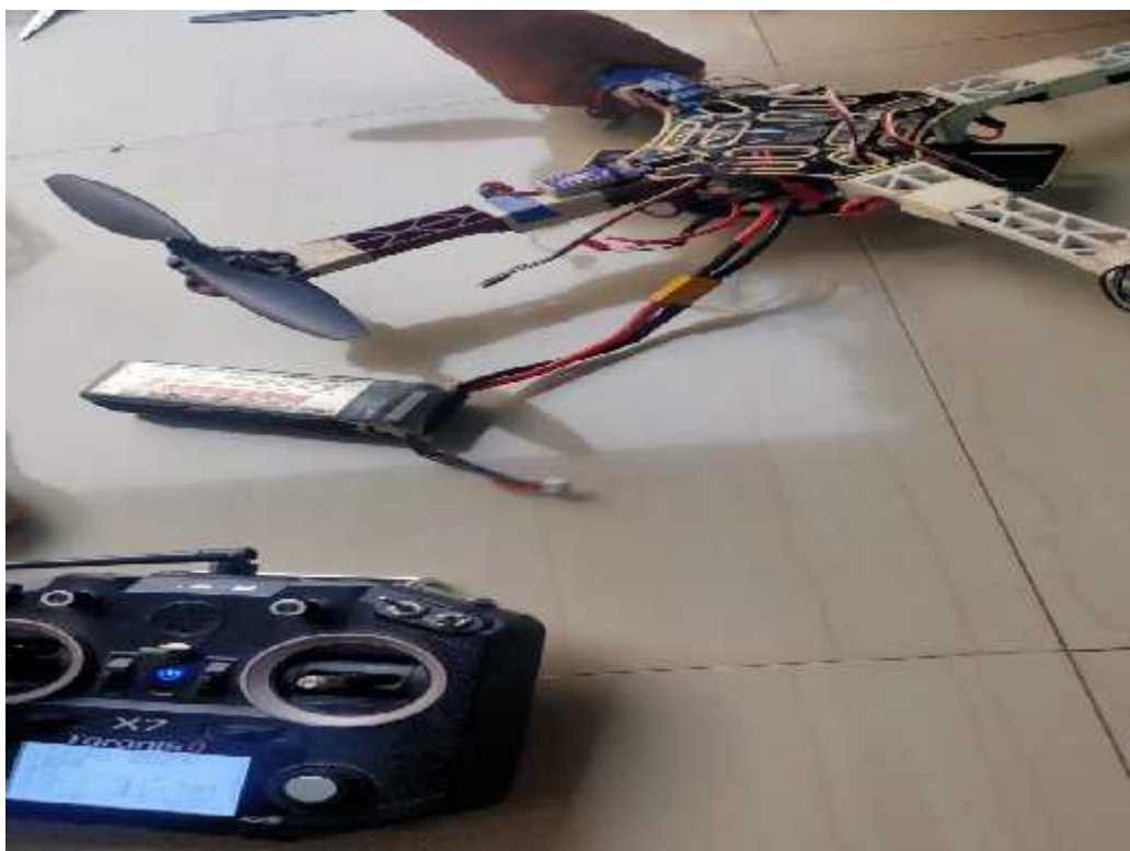
Gambar 4.5 kalibrasi Electrical Speed Control (ESC)
