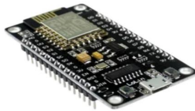
Gambar 2.2. NodeMCU ESP8266 (Nurul Hidayati Lusita Dewi dkk, 2019)
