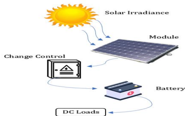
Gambar 2.2 PLTS Off Grid
