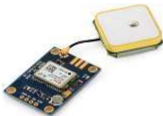
Gambar 2.3 Modul GPS Ublox Neo 6M (Sumber : https://www.nn-digital.com )
