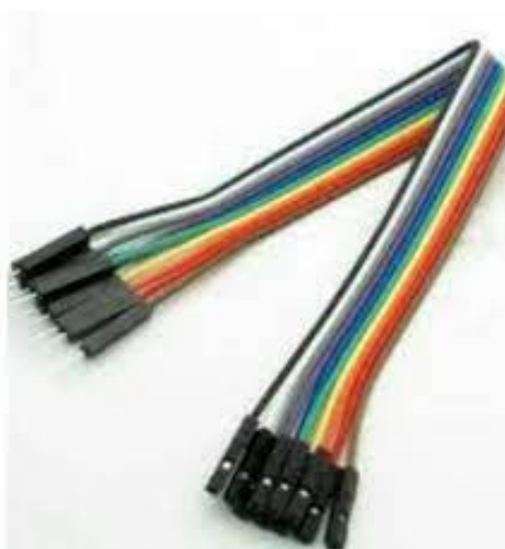
Gambar 2.7 Kabel Jumper Sumber: (Ipanhar et al., 2022)
