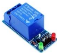
Gambar 2. 11 Module Relay Sumber : (Safi'i, 2022)
