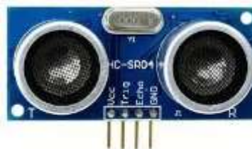
Gambar 2.4 Sensor Ultrasonik (Elga Aris Prastyo, 2022a).
