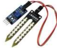
Gambar 2.3 Sensor soil moisture (Haris & Algorista, 2020).
