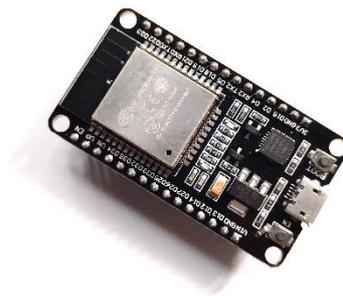
**Gambar 2.3** Modul NodeMCU ESP32
