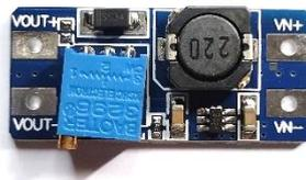
**Gambar 2.7** Modul MT3608 DC-DC *Step Up*
