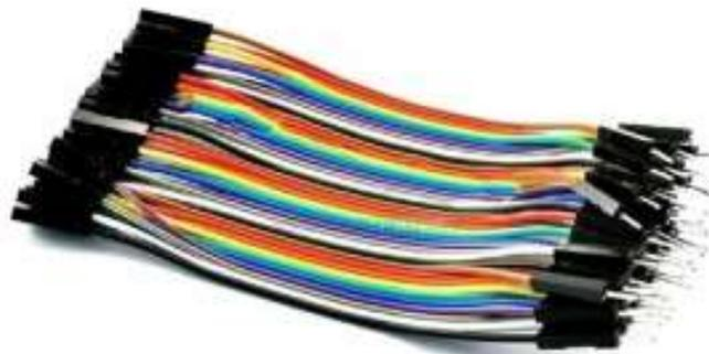
Gambar 2. 2 Kabel Jumper
