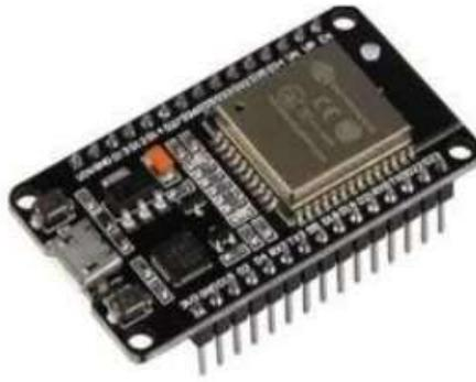
**Gambar 2.5** NodeMCU ESP32
