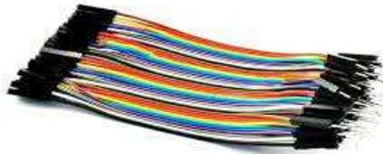
**Gambar 2. 9** Kabel Jumper
