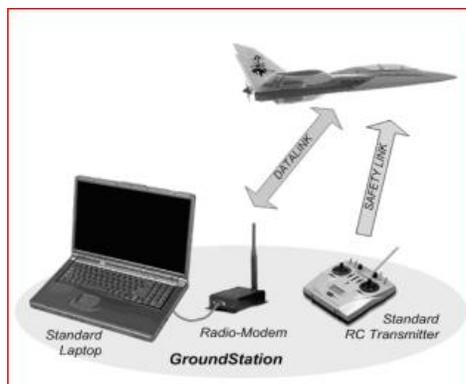
**Gambar 2.2** Sistem *Unmanned Aerial Vehicle (UAV)* Secara Umum
