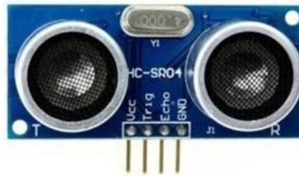
**Gambar 2.2** Sensor Ultrasonik
