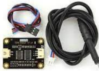
Gambar 2.8 Sensor TDS Meter Sumber : (Aldy Razor, 2022)
