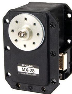
**Gambar 2. 1** Aktuator Dynamixel Tipe MX-28T
