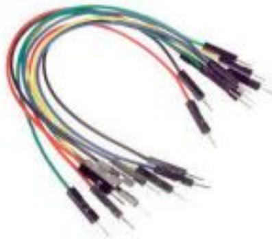
**Gambar 2.6** Kabel Jumper
