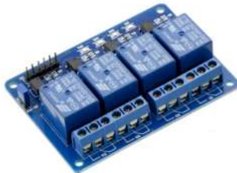
Gambar 2.8 Relay (Sumber: https://core-electronics.com.au/5v-4-channel-relay-module-10a.html )
