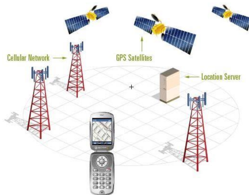
Gambar 2.1 Cara kerja Global Positioning System (GPS) http://www.navigadget.com/wp-content/postimages/2007/01/a-gps-944.jpg
